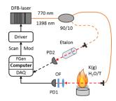
The **Applied Laser Spectroscopy Group** develops laser-based spectrometers and techniques for fast and accurate detection of atomic and molecular species in gas-phase. The sensors are employed in applications such as real-time in situ combustion diagnostics and detection of biomarkers in exhaled breath for medical diagnostics.
